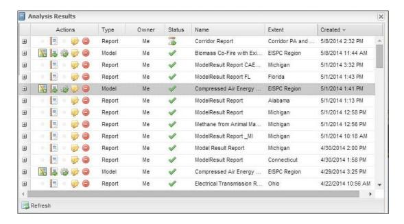
When the **Analysis Results** window is open, the hour glass icon in the **Status** column indicates that the model or report is running, and a checkmark icon indicates it is complete. Hovering the cursor over the **Actions** icons will reveal **tool tips** about their functions, and clicking on the **Actions** icons will run them. The icons include:
