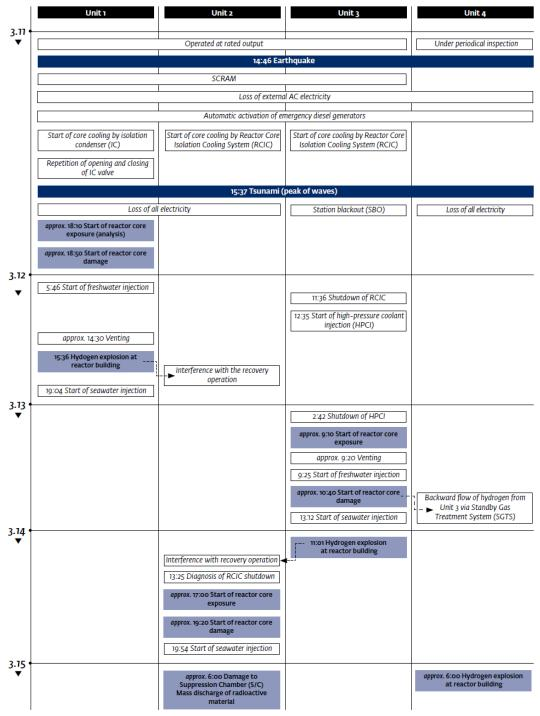
°Start of reactor core exposure and start of reactor core damage times are both from TEPCO's MAAP analysis results.
