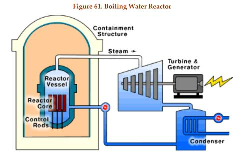
The boiling water reactor (BWR) was designed by General Electric (GE-Hitachi) to compete with Westinghouse's PWR design. Advantages to the BWR include operating at a lower pressure removes the need for a high pressure reactor vessel and direct transfer of reactor steam to the steam turbine eliminates the need for the steam generator found on PWRs. One drawback is that BWR operators are exposed to higher radiation levels.
