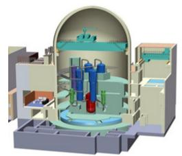
A four-train redundant safety system provided to enhance safety and improve reliability. NRC design certification for the U.S. APWR is underway and currently projected for completion in 2015. In the meantime, both Dominion Energy (North Anna) and Luminant (Comanche Peak) have COL applications before the Nuclear Regulatory Commission.<sup>228</sup>
